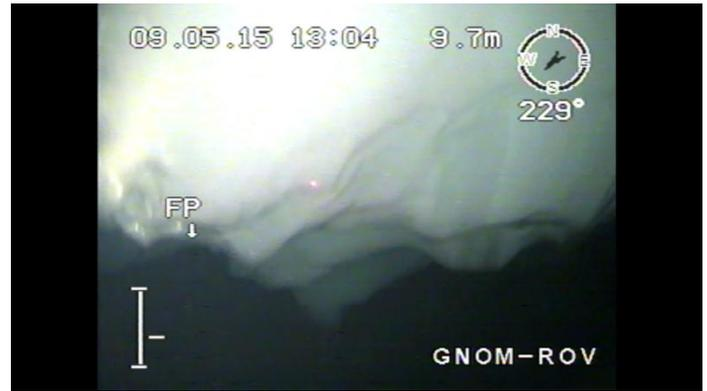
Fig. 5 - Video filming of the ice ridge keel using the ROV "Gnom"
