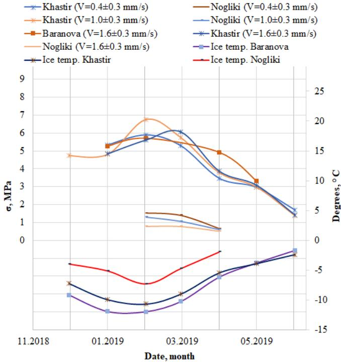
Fig. 12 – Uniaxial compression strength and ice temperature at all bases.
