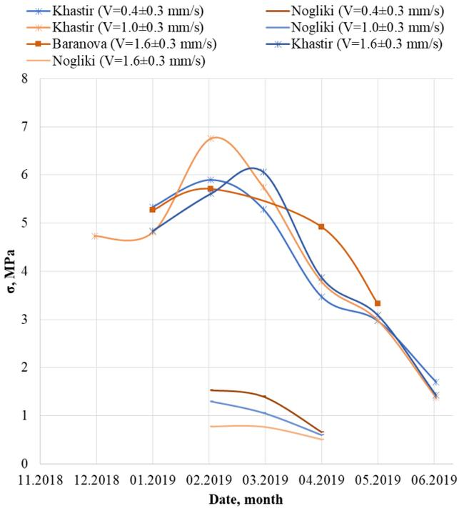
Fig. 9 - Uniaxial compression strength of samples drilled parallel to the surface of the ice sheet at different loading velocities for all bases.
