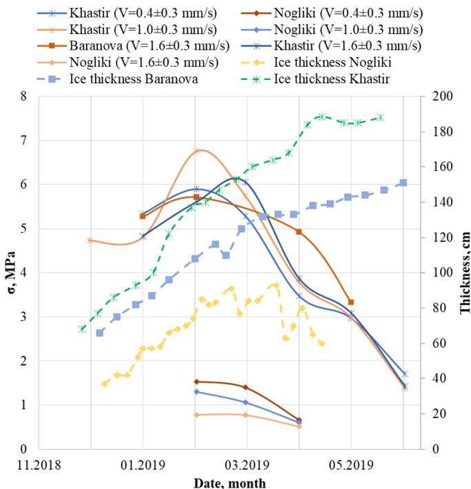
Fig. 13 - Uniaxial compression strength and thickness of ice for all
