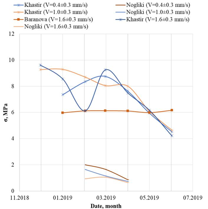
Fig. 8 - Uniaxial compression strength of samples drilled perpendicular to the surface of the ice sheet at different loading velocities for all bases.
