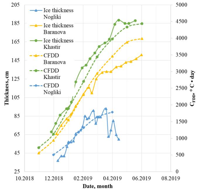
Fig. 11 - Sum of degree-days and thickness of ice for all bases.
