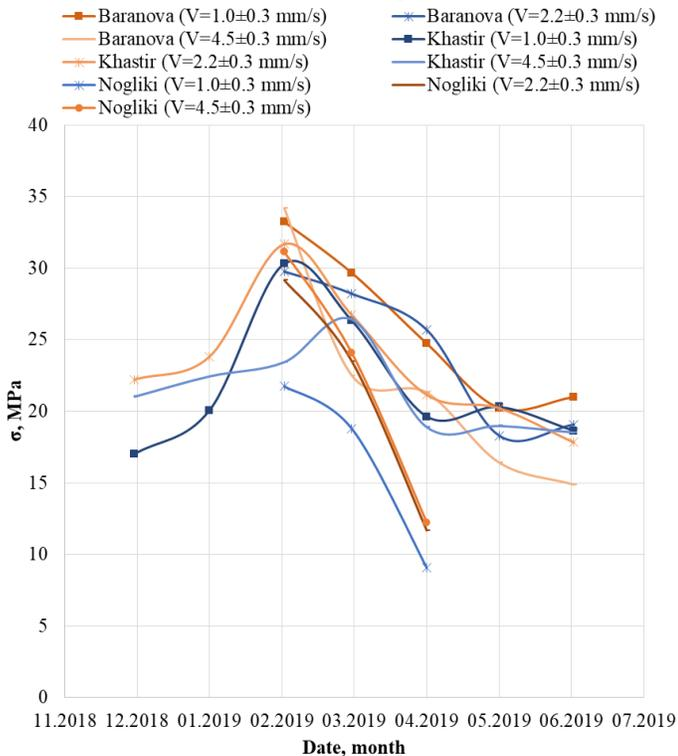
Fig. 10 - Borehole jack ice strength at different loading velocities for all bases.
