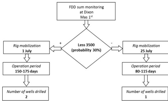
Fig. 7. Decision tree for exploration drilling with ice-resistant platform on the structures of the first group.
