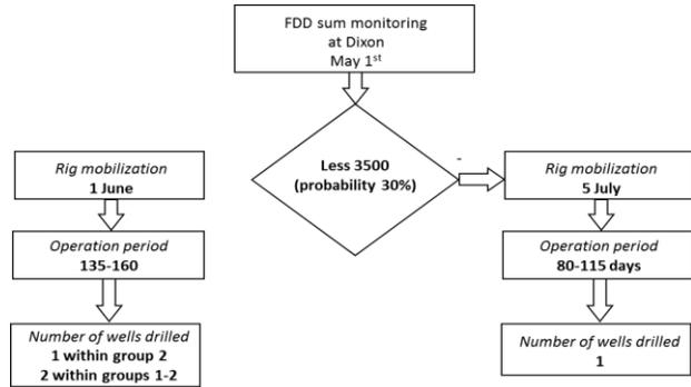
Fig. 8. Decision tree for exploration drilling with ice-resistant platform on the structures of the second group.
