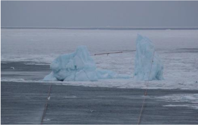
Fig. 4. Iceberg #12 after course change by 90°. Rope raise-up
